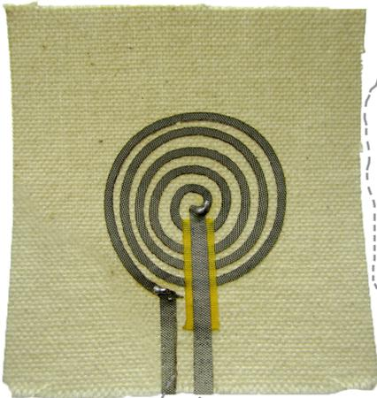
It's not just for clothing though. Researchers at MIT made an interactive wall that uses conductive paint to make touch sensors work with lights and motors magnetically attached to the wall, all while looking like a beautiful mural! In another project, they put a variety of flexible conductive materials on paper or fabric in a spiral to make an electromagnet. When an audio signal is run through it, it acts just like a regular speaker, but flat and soft!
